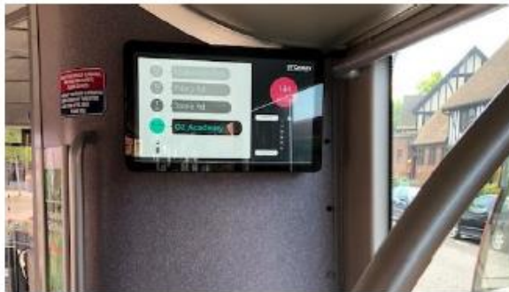
Example of accessibility screens installed in Worcestershire buses
